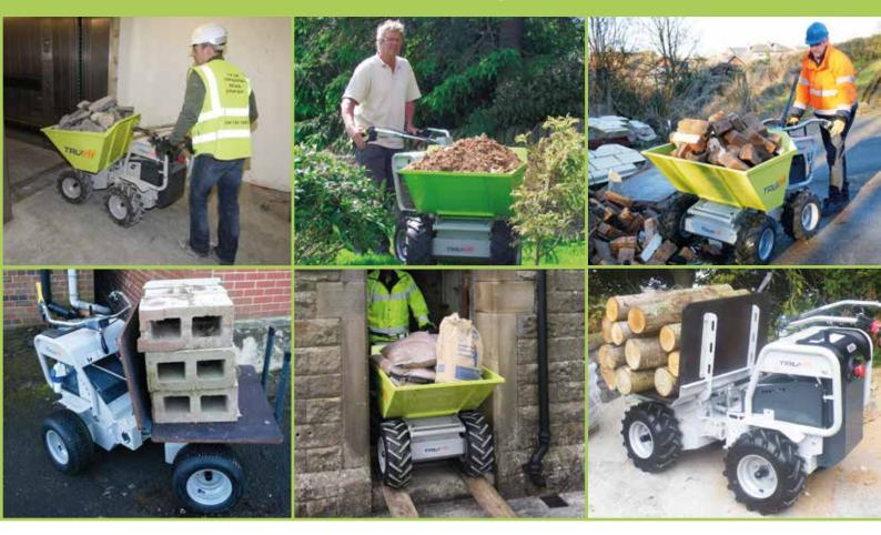
**300 BENDie** - 300kg (660lbs) payload, articulated **450 BENDie** - 450kg (990lbs) payload, articulated
